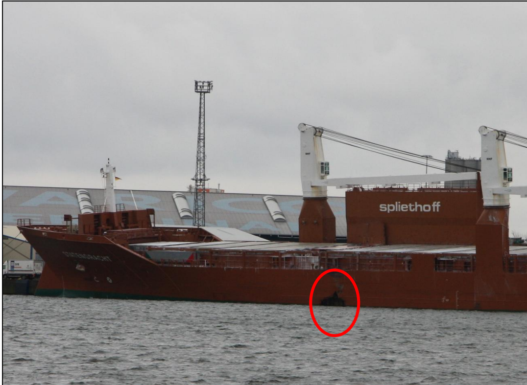
Figure 15: Damage to Statengracht 's side shell plating
